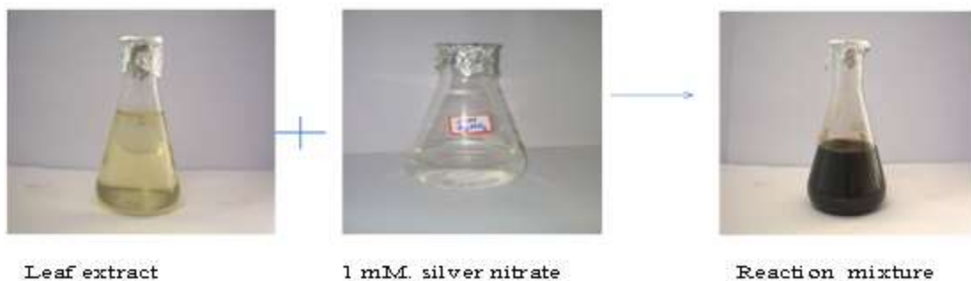
Fig. 2 Change in colour of reaction mixture due to formation of silver nanoparticles.
