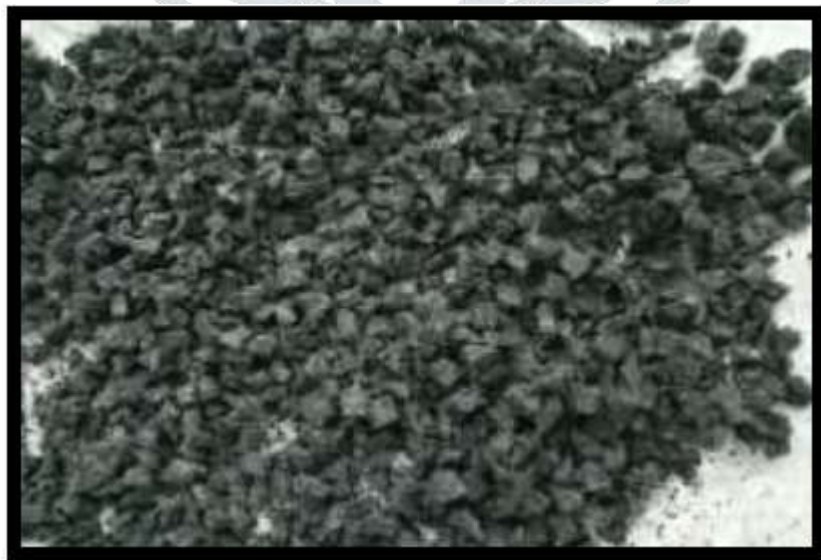
Fig. 3 Physical appearance of plastic waste blended with \text{Na}_2\text{SiO}_2
