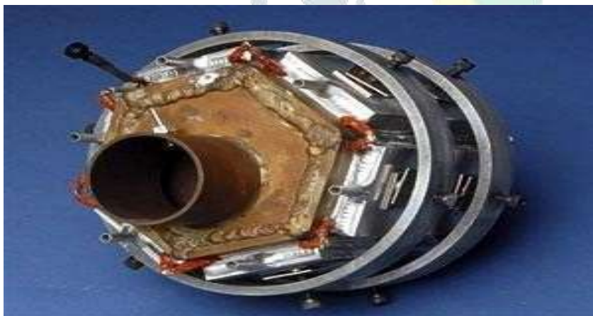
Figure 9- thermoelectric generator used in vehicle
