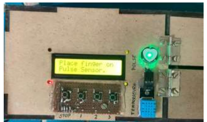
Fig.3 LCD Showing the Pulse sensor operation
