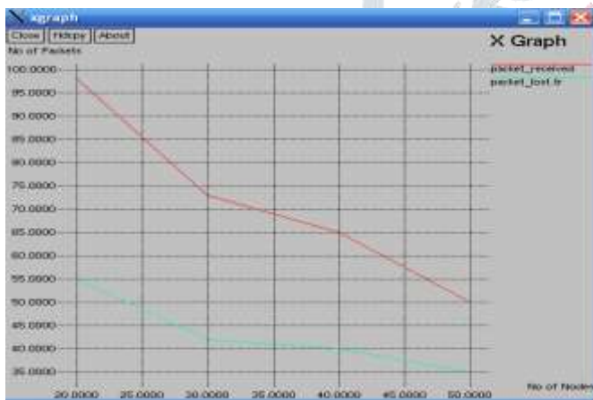
Fig. 7. Packet rate with black hole node in IDSAODV
