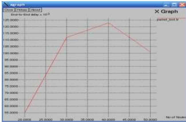
Fig. 13. Packet lost for E2E delay in the AODV protocol with the blackhole node
