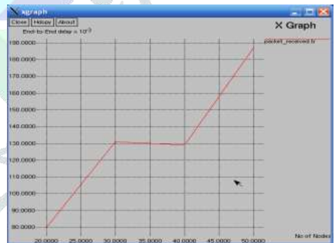
Fig. 12. Packet received for E2E delay in the AODV protocol with no blackhole node
