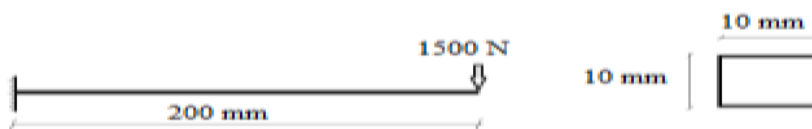
Figure 2. Cantilever Beam with Tip Point Load
