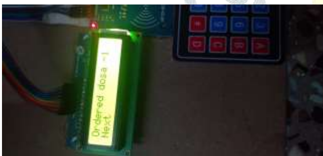
Fig.9: LCD Showing the ordered menu to the kitchen section once order given by the customer
