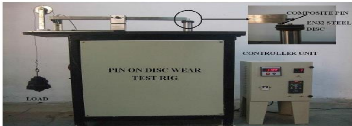
Fig :Pictorial view of Pin-on-Disc wear test rig
