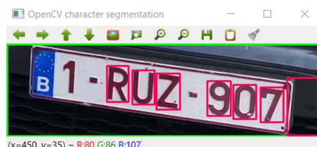
Fig. 10: Result for OpenCV character Segmentation window displaying the coordinate values.
