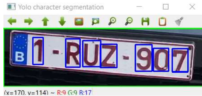
Fig. 11: Result for YOLO character Segmentation window displaying the coordinate values.
