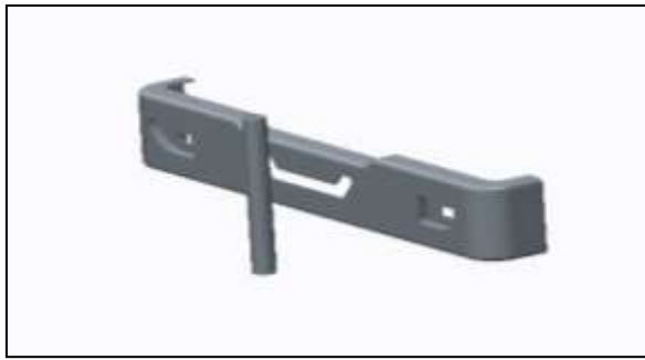
Figure 2: Assembly model of bumper and legform at 250mm from ground
