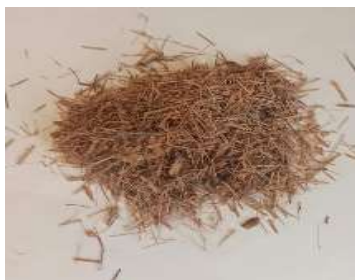
Fig 3 Coconut Coir Fiber used in reinforcement phase
