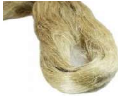
Fig. 4 Sunn Hemp Fibre used in reinforcement phase
