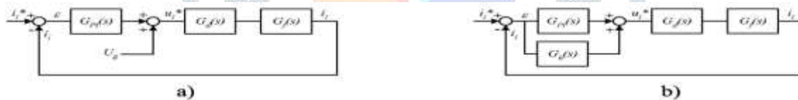
Fig 6 : The current loop of PV inverter: a) with PI controller; b) with PR controller.
