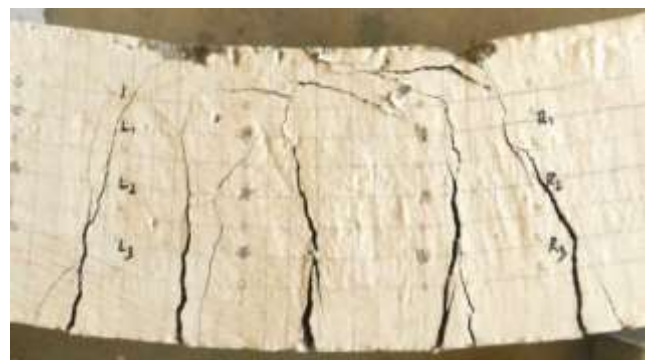
Beam failure pattern
