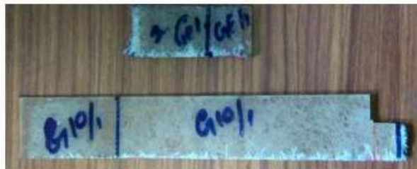
Fig no 2 GF 10 % and PR 90 % by volume composite
