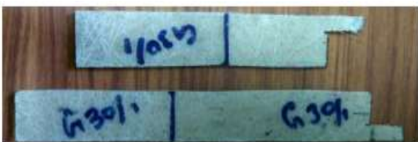
Fig no 4 GF 30 % and PR 70 % by volume composite
