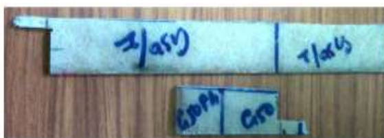
Fig no 6 GF 50 % and PR 50 % by volume composite
