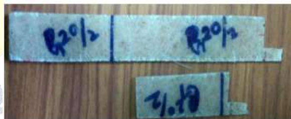
Fig no 3 GF 20 % and PR 80 % by volume composite
