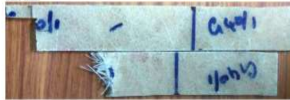
Fig no 5 GF 40 % and PR 60 % by volume composite
