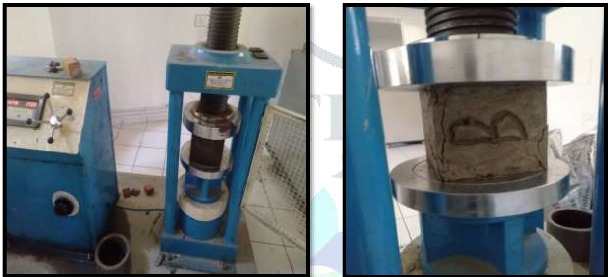
Fig.2 Compressive strength test on concrete block
