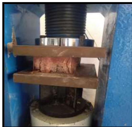
Fig. 1 Compressive strength test on paver block
