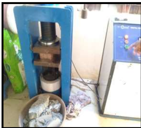
Fig. 1 Compressive strength test on paver block
