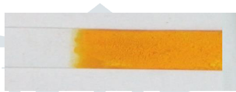
Fig.2: Double layer CdS-(Cd 0.8 Zn 0.2 )S nano film.
