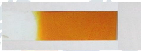
Fig.3: Multilayer CdS-(Cd 0.8 Zn 0.2 )S-(Cd 0.5 Zn 0.5 )S thin film.
