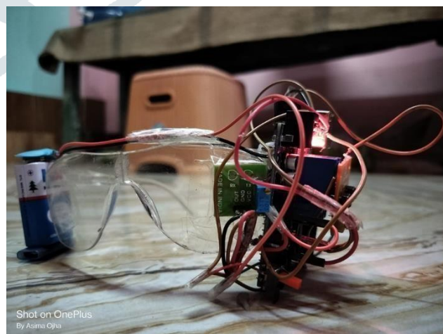
Figure 6. Eyeglass With the Eyeblink Sensor
