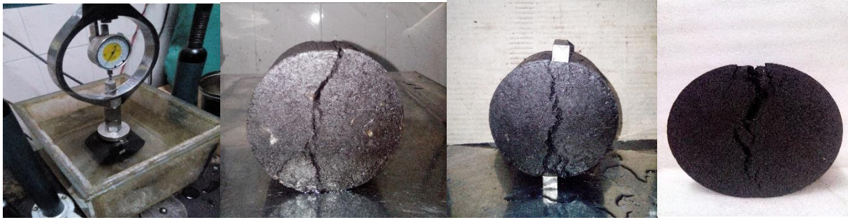
Figure 4.7 Loading And Failure Pattern of Indirect Tensile Strength Test.
