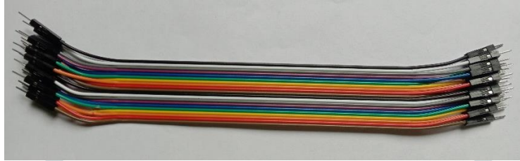
Figure No.06 : Connecting Wires
