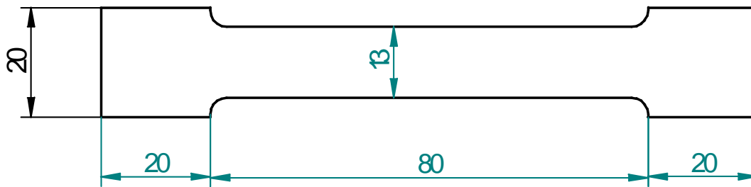
Fig.5.4 Dimensions of Tensile test specimen in “mm”
