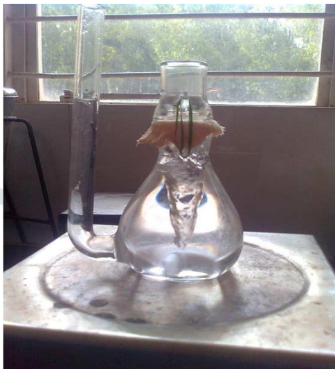
Fig 1: Franz diffusion cell with skin mounted between compartments
