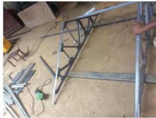
Fig 5.2 Assembling the members
