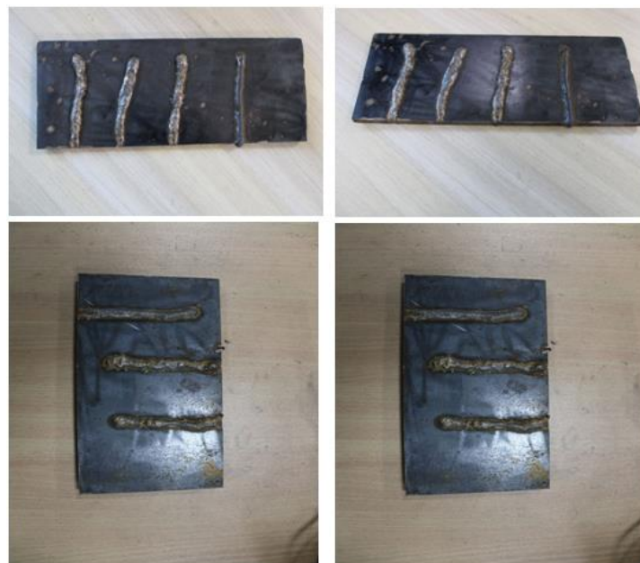
Figure 1. Weld beads achieved during the welding process
