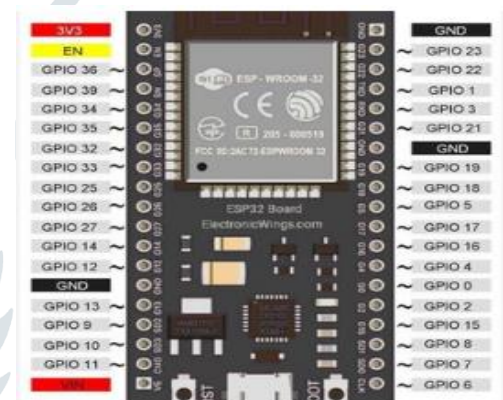
Fig. 1. Pin diagram of ESP32 Microcontroller
