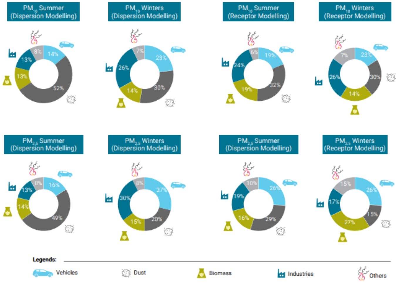
Fig 5.1 Sectoral Share estimated by Dispersion Modelling and Receptor Modelling. Source: ARAI and TERI (August 2018)
