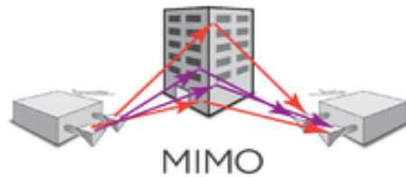
Fig.2. (a) MIMO uses Multipath propagation to exploit link capacity. (b) SM system model.
