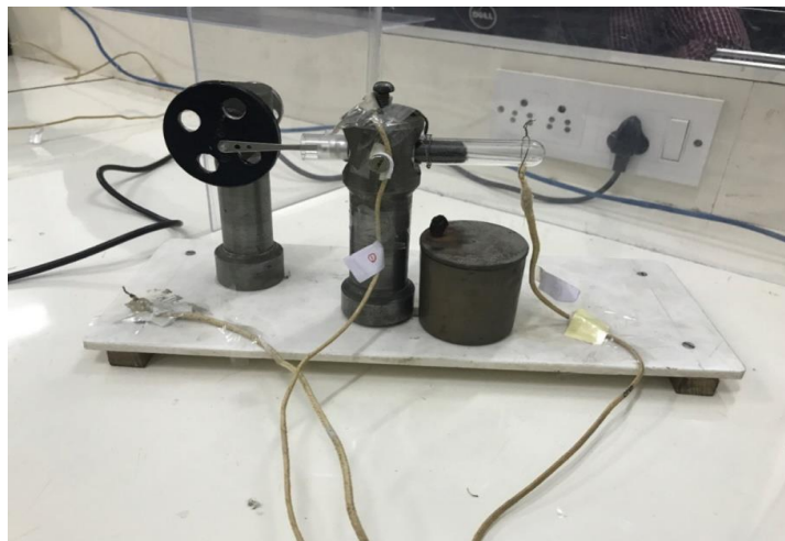
Fig 2: Actual Image of Thermoacoustic Engine
