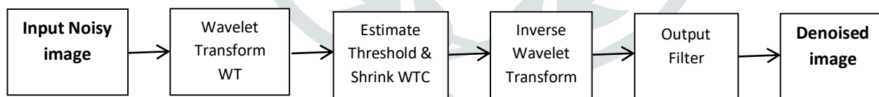
Figure1. Block diagram of Image denoising using Wavelet Thresholding
