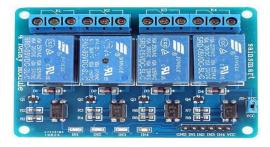
Figure 3: Relay Module
