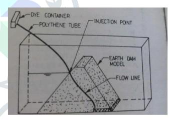
Fig. 3 – General layout of model.
