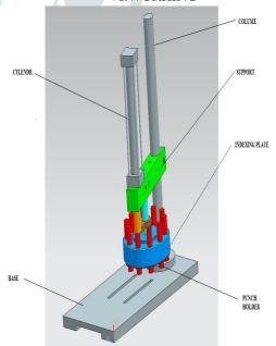
Figure:3D View of Assembly of Pneumatic Punching Machine
