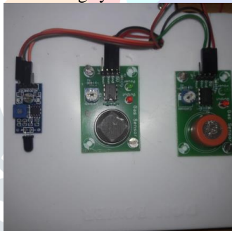
Fig. 8 The Fire, Gas and alcohol sensors mounted at the top of the tracking system
