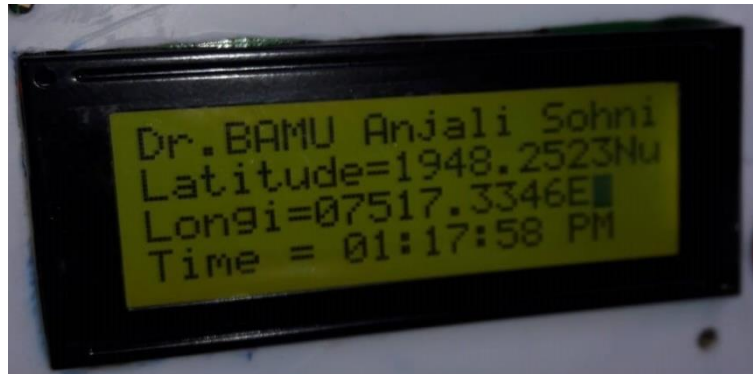
Fig.7 The LCD display on the vehicle tracking system showin realtime location parameters
