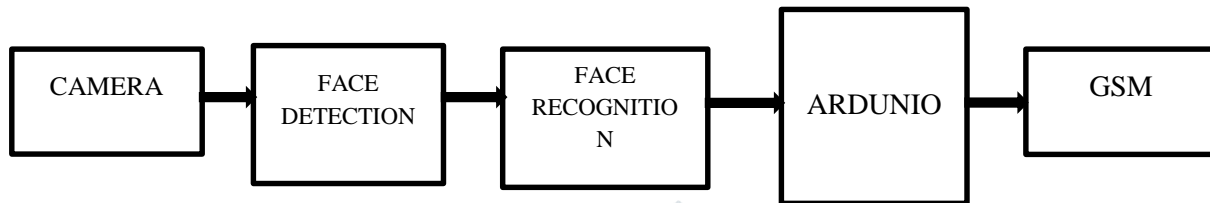
Fig1 Block Diagram of Proposed System
