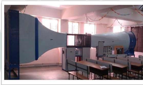
Figure 4: Low speed wind tunnel facility
