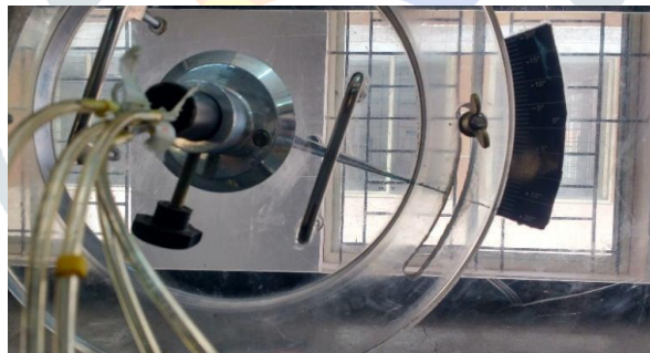
Figure 7: Model at 15° Angle Of Attack
