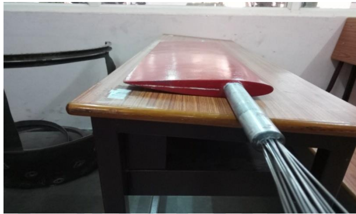
Figure 6: Fabricated Model Of The Wing.
