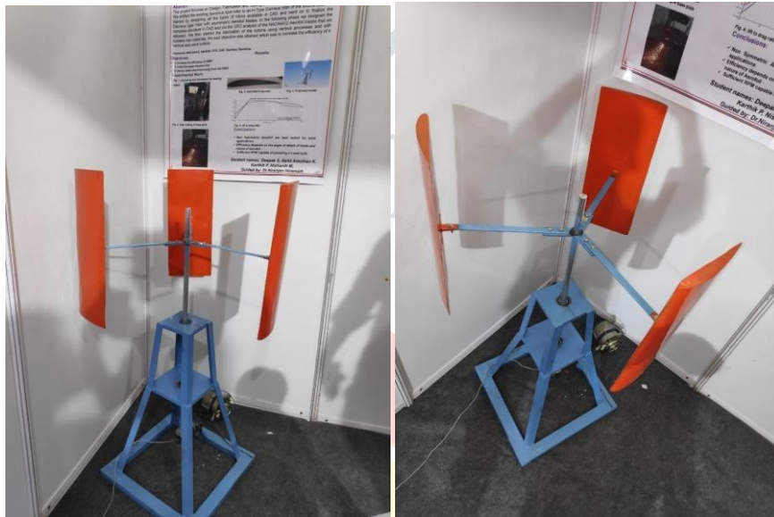
Figure 7.4 Assembled model of the proposed VAWT
