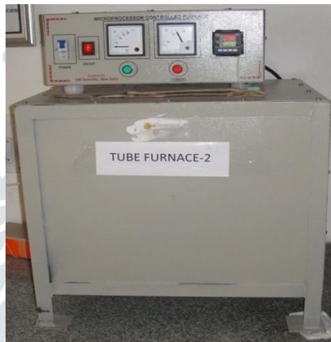
Figure 2.1 Hot corrosion Experimental setup
