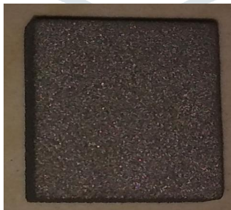
Fig 3.3 Macrograph of coated sample WCNi+NiCr
