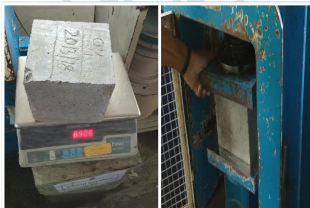
Fig No. 4 Compressive Testing on CTM
