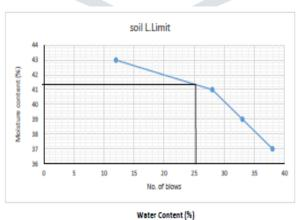
Figure 4.1 liquid limit for soil
