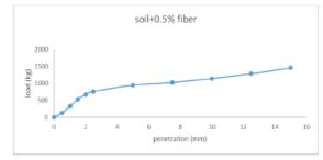
Figure 4.18 soil reinforced with 0.5 % coir
