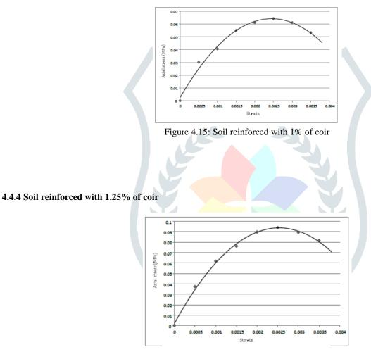
Figure 4.16: Soil reinforced with 1.25% of coir
