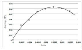
Figure 4.13 soil reinforced with 0.5 % coir
