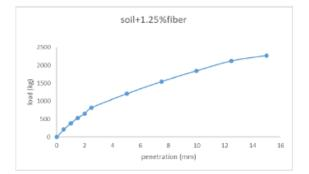
Figure 4.21: Soil reinforced with 1.25% of coir
