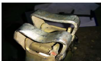
Fig.6.Failure of jack head due to improper design
