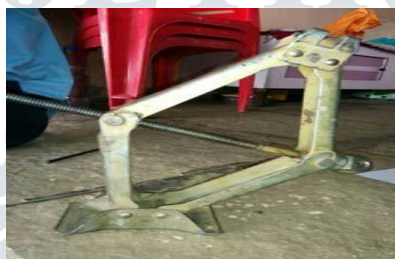
Fig.4 Toppled scissor jack due to arm teeth failure
