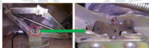
Fig. 5 Failure of screw and arm teeth
