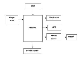
Figure 1 vehicle tracking system with finger print
