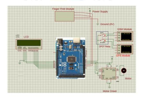
Figure 4 Main circuit diagram of proposed system
