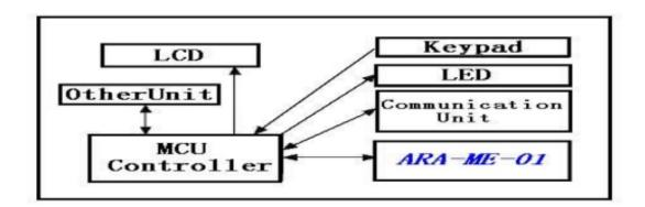
Figure 3 MCU controller diagram
