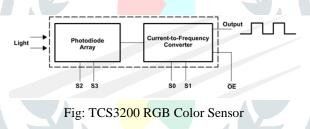
The TSC3200 Color Sensor IC is an 8 pin IC with SOC package. The following image shows the pin diagram of the Color Sensor IC. In that Pins 1 and 2 (S0 and S1) are output frequency scaling pins. Pin 3 is Output enable pin and is an active low pin. Pin 4 is GND.
