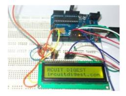
Fig: 16×2 LCD Interfacing with Arduino Uno
