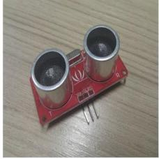
Fig 2: Ultrasonic sensor
