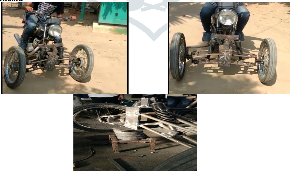
Fig (7): Front A-arm attached to wheel hub
