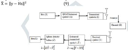
Fig-4: Flow Diagram of Sphere Decoder
