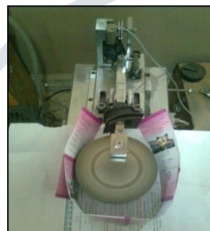
Fig 1: Pin on disc testing Fig 2 : Micro- balance weighing machine
