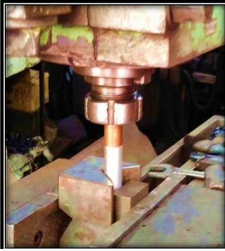
Fig.1. Experimental Set-up of the Friction Welding process
