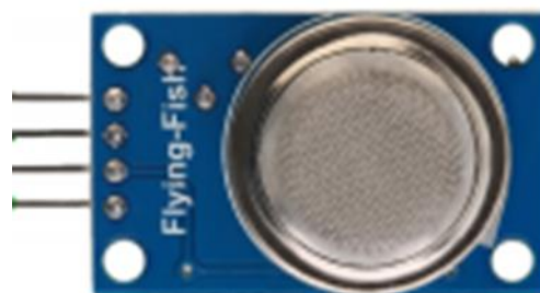
Fig. 7. Carbon Monoxide Sensor
