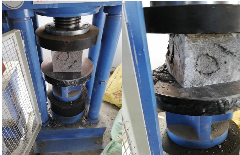
Fig. 2 (A) Before compression test on specimen (B) After compression test on specimen
