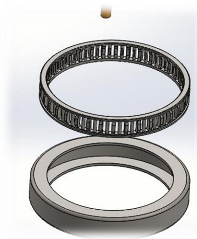
Fig. 2 Part Assembly of Needle Roller Bearing
