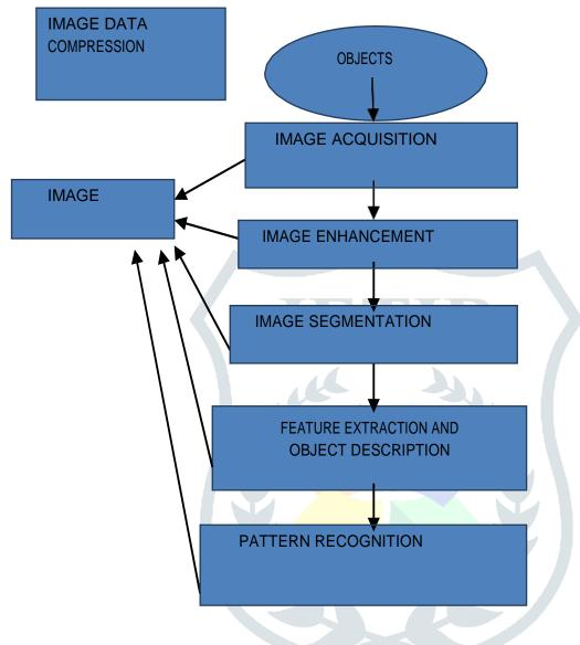
Fig: The Basic Steps of Image Processing
